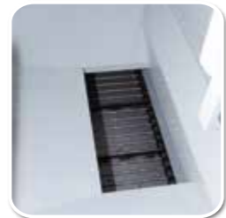
Drainage outlet & Chip conveyor
